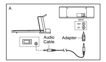
B. Plug one end of the audio cable into the jack on the front of the treadmill near the power cord. Plug the other end of the cable into the LINE OUT jack on your stereo.
